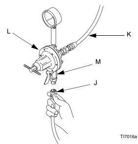
Fig. 9: Connect Fluid Hose
